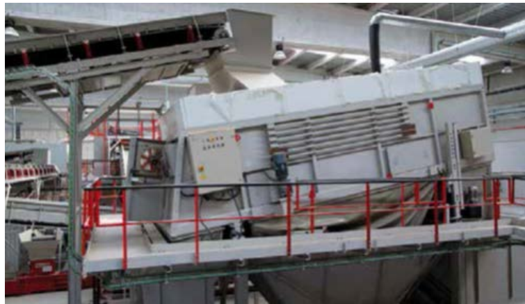
Figure 26 Classification using a ballistic separator based on density in segregating light flat material (film and P/C) from heavy rolling material (packages). (Source: ECOEMBES, 2021)
