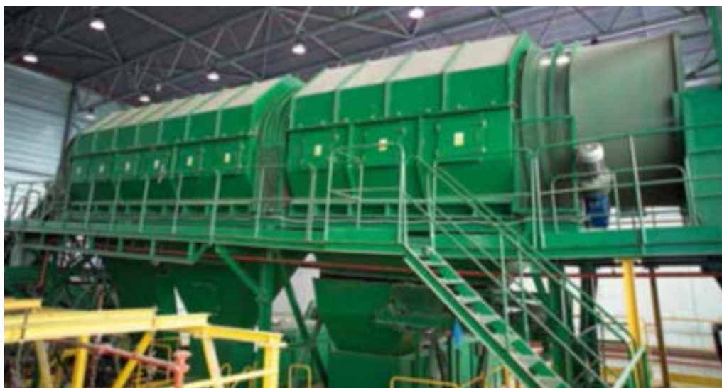
Figure 25 Classification in trommel by size to separate lightweight packaging (underflow) from organic matter (fine waste underflow) and bulky waste (overflow). (Source: ECOEMBES, 2021)
