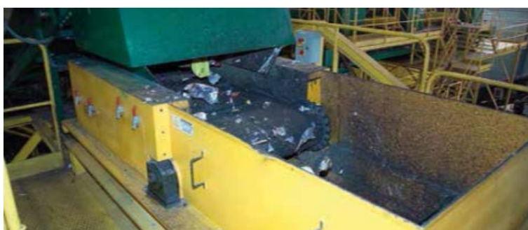
Figure 28 Induction separators remove aluminum material using eddy currents. (Source: ECOEMBES, 2021)
