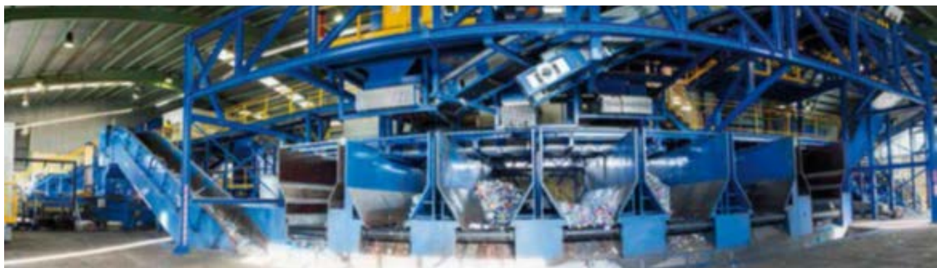
Figure 21 Lightweight packaging sorting plant. (Source: ECOEMBES, 2021)
