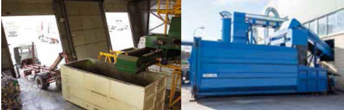
Figure 31 The rejected waste material at the facility is compacted or stored in containers for delivery to the landfill site.
