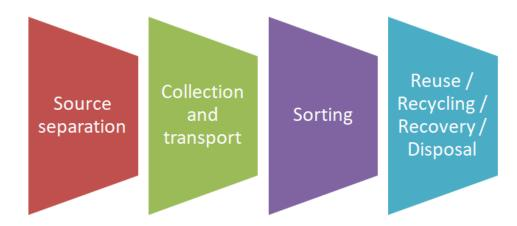
Figure 15 Elements in a waste management system
