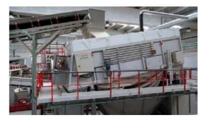
*Figure 26* Classification using the ballistic separator based on density in segregating light-flat material (film and P/C) from heavy rolling material (packages). (Source: ECOEMBES, 2021)
