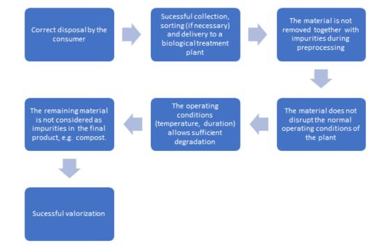
Figure 34 An example of a possible route of valorizing compostable plastics through biological treatment
