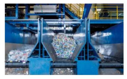
Figure 30 Temporary storage of selected materials. (Source: ECOEMBES, 2021)
