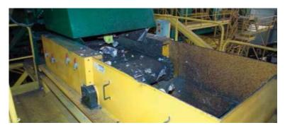
Figure 28 Induction separators remove aluminium material using eddy currents. (Source: ECOEMBES, 2021)
