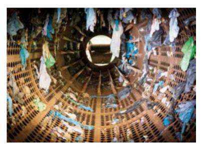
*Figure 32* Classification Trommel: Divides the material stream into two or more categories according to grain size using specific size sieves. (Source: ECOEMBES, 2021)
