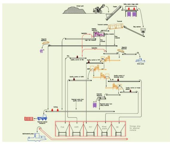
Figure 23 Diagram of the automated sorting process. (Source: Elaborated by ECOEMBES, 2021)
