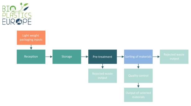
Figure 22 Outline of sorting process. (Source: Elaborated by ECOEMBES, 2021)
