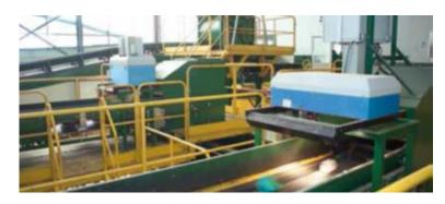
Figure 27 Optical separators. (Source: ECOEMBES, 2021)
