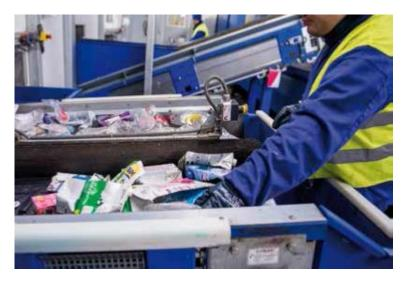
Figure 29 Quality control of selected materials. (Source: ECOEMBES, 2021)
