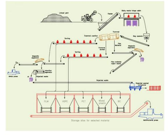
Figure 24 Diagram of the manual sorting process. (Source: Elaborated by ECOEMBES, 2021)
