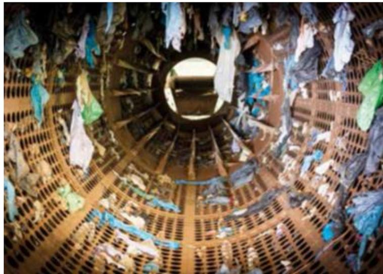
**Figure 32** Classification Trommel: Divides the material stream into two or more categories according to grain size using specific size sieves. (Source: ECOEMBES, 2021)
