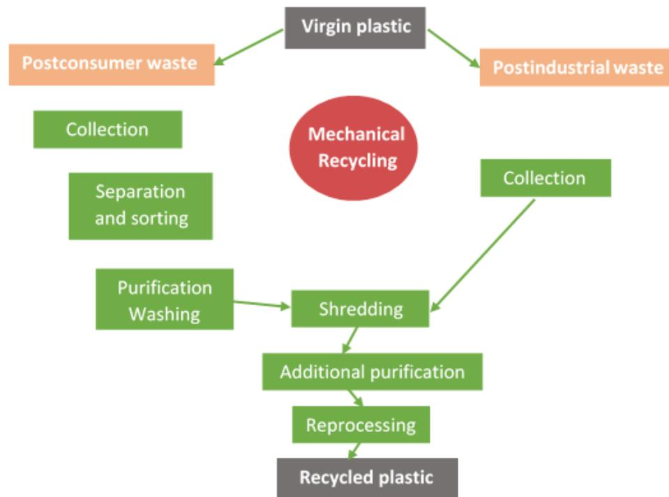
Figure 33 Stages of the mechanical recycling process.
