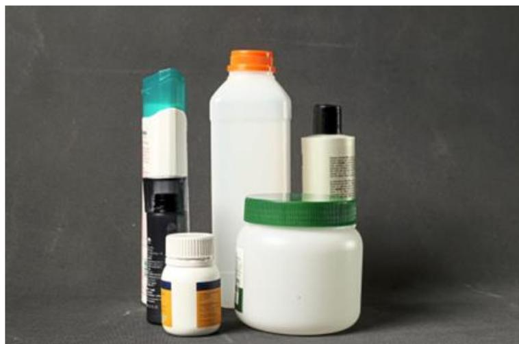
*Figure 5 High-Density Polyethylene (HDPE) Photo: The Star/Azman Ghani*
