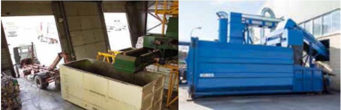
*Figure 31* The rejected waste material at the facility is compacted or stored in containers for delivery to the landfill. (Source: ECOEMBES, 2021)
