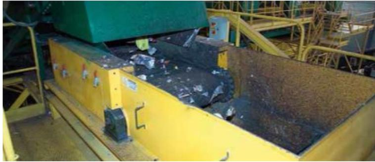
*Figure 28 Induction separators remove aluminium material using eddy currents. (Source: ECOEMBES, 2021)*
