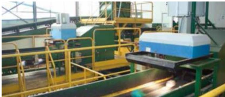
*Figure 27 Optical separators. (Source: ECOEMBES, 2021)*
