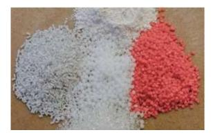
NaturePlast produces a range of biocomposites containing natural fibres or by-products from different activities
